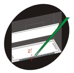
6. Using the tweezers again, use it to lift out the focusing screen by grabbing onto either tabs on the side of the focusing screen. Lift it out slowly in the same manner how you did with the metal bracket (albeit lifting it an angle will be slight more difficult as the small tab is being held by the tweezer). Note how the focusing screen is pulled out as you'll want to ensure you put it back in the same way (and not upside down or reversed).
