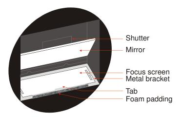
5. Using a small tweezer, grip the little metal tab with the tweezer and push the tab gently towards the back of the camera (1) then lift up (2) as shown below. The metal bracket should pop up. This does not take a lot of force to accomplish. When lifting the metal bracket, ensure that it is firmly held and pulled away from the mirror to prevent scratches on the mirror.
